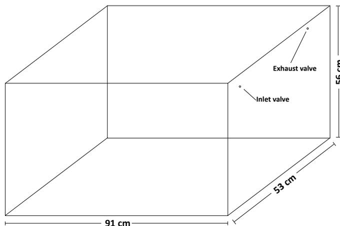
**Figure 1. Example dimensions of a box for suckling pigs with inlet and exhaust valves indicated.**
