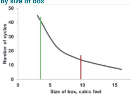
Maximum box size for a 50% box volume exchange rate, if box is equipped with a single 125 CFH flow meter. Up to 8 small suckling pigs may fit in a box this size, \$0.05/pig
