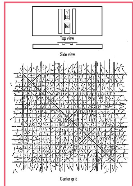
**Figure 6. Diagram of both top and side views of a hemacytometer, and the center grid area where sperm are counted in order to estimate sperm concentration.**
