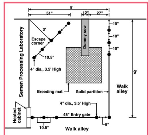
**Figure 2. Schematic of an on-farm semen collection pen. Notes: 1. If young boars walk between the escape pipe, place larger diameter pipe over the smaller pipe until boars get larger. 2. A pig board is kept in the escape corner.**
