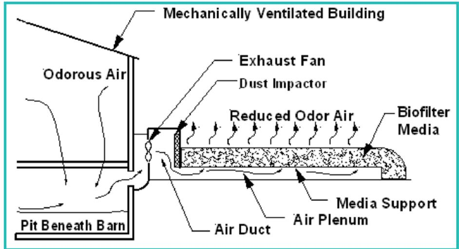
Figure 2. Schematic of a typical open-faced biofilter
