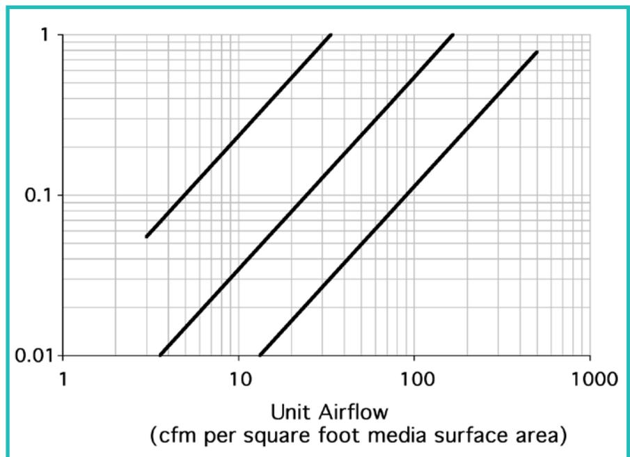
Figure 4. Media unit pressure drop and unit flow rate relations for various biofilter media.
