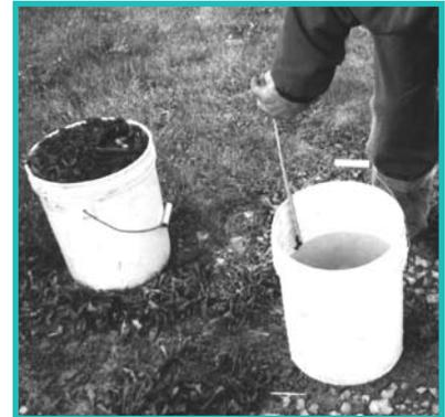
Figure 6. Step 8 measuring water removed
