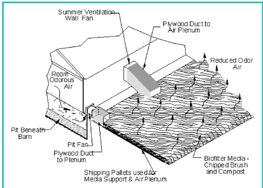
Figure 8. Biofilter construction
