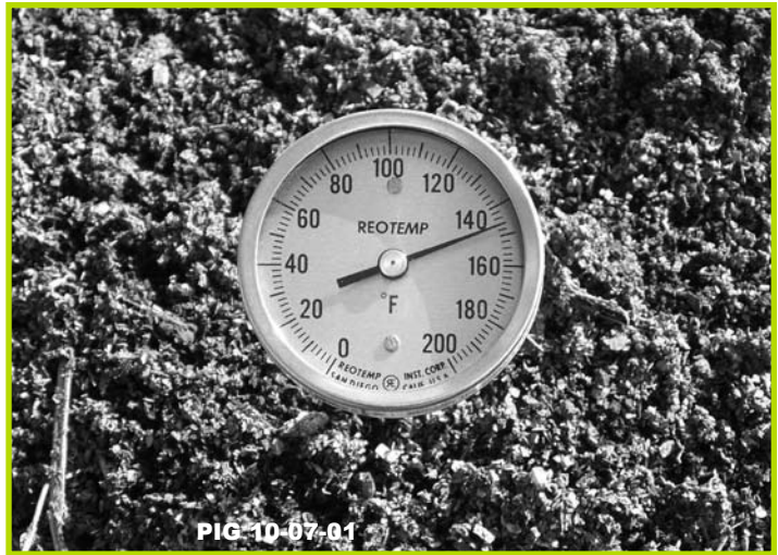
Composter thermometer with 36 inch shaft inserted into an active compost pile.
