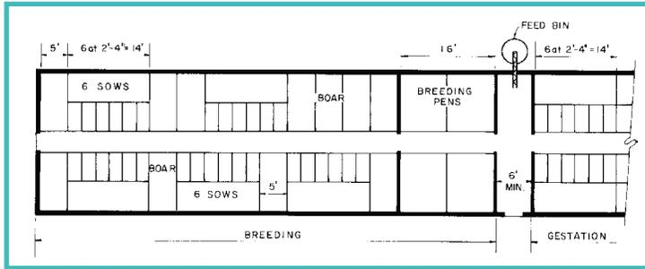
Figure 6. Partially slotted-floor gestation and breeding building.
