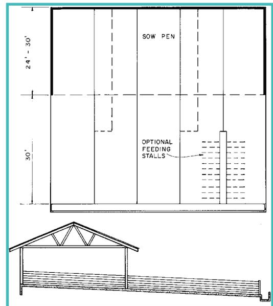
Figure 2. Open-front shed with an outside run.
