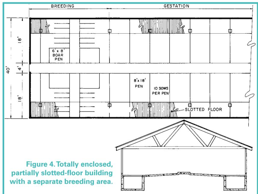
Figure 4. Totally enclosed, partially slotted-floor building with a separate breeding area.
