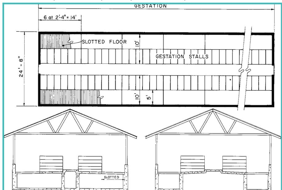
Figure 5. Partially slotted-floor gestation building, with alternative floor construction.
