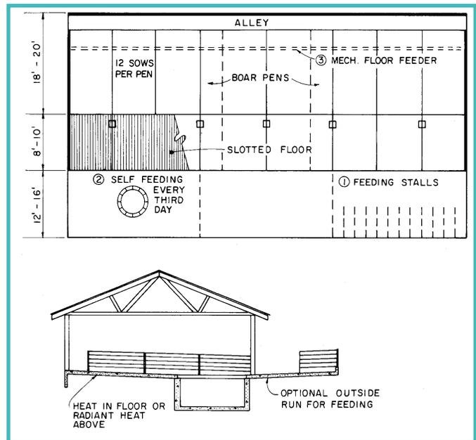
Figure 3. open-front, partially slotted-floor building.
