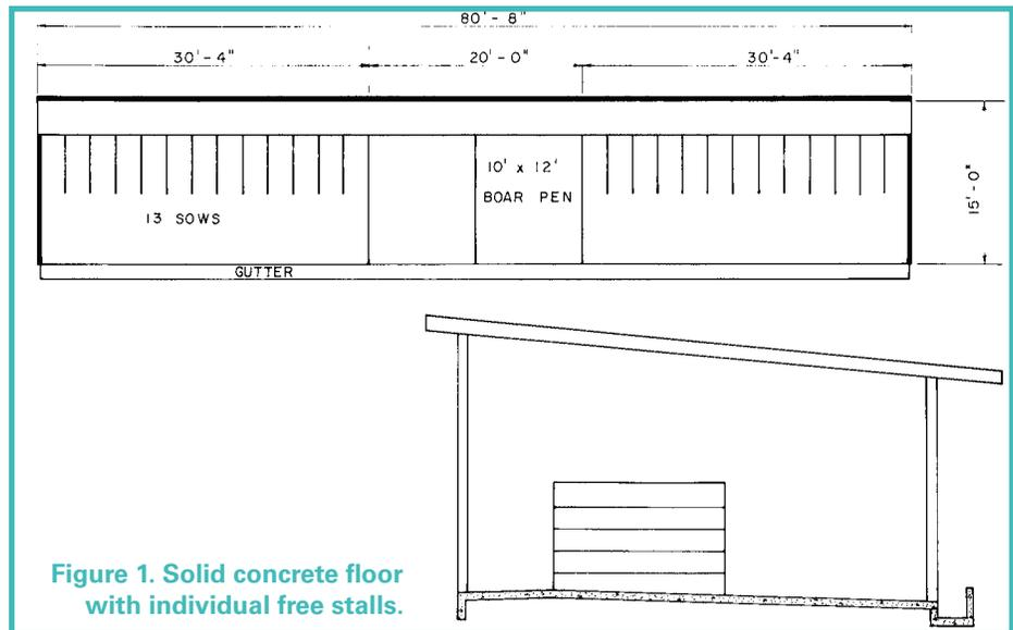
Figure 1. Solid concrete floor with individual free stalls.
